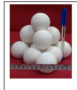
Pressure cast and sintered to >98 density
